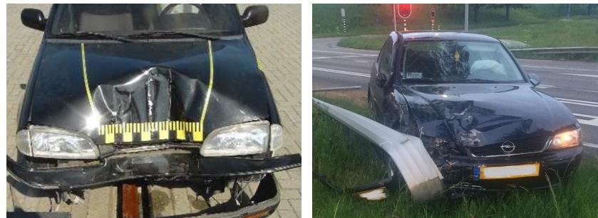
Picture left: picture of an official crash tested car according EN12767 where the impact point on the test vehicle shall be centered to be within \pm 0,1m .
